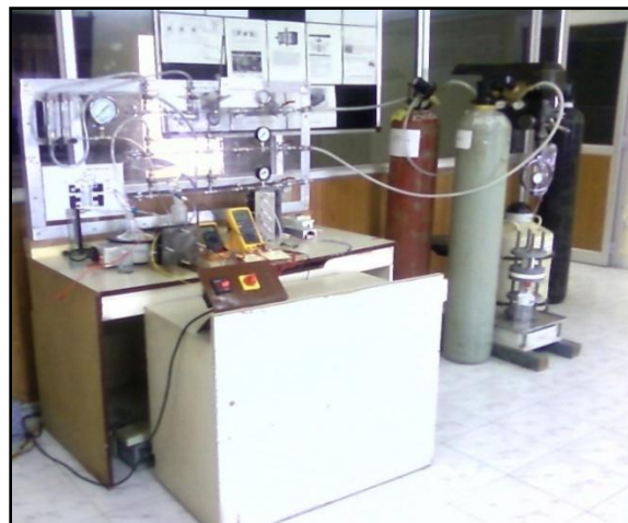
Figure 8 Shows single cell being tested on fuel cell test station
